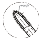
BA 114/T Aspiration Handpiece, smooth abrasive (rough) tip, (0.65mm) Asp. port 0.30 mm
