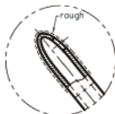
BA 119/T Special model Aspiration Handpiece, smooth abrasive (rough) tip, (0.70mm) Asp. port 0.35 mm
